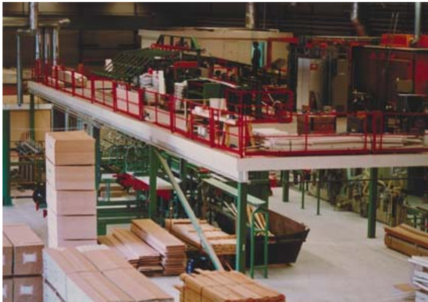
Fig. 9: Installation for boarder materials. (2 x 180 kV, 30 mA, 300 mm)
