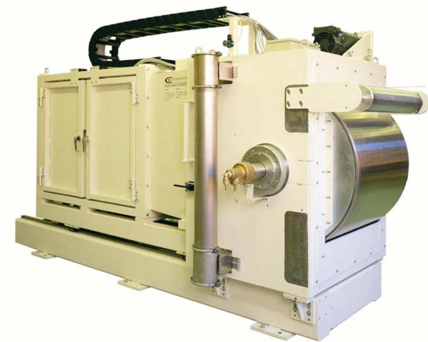
Fig. 15: EB unit for irradiation of material from roll to roll. (120 kV, 220 mA, 0,6 m)
