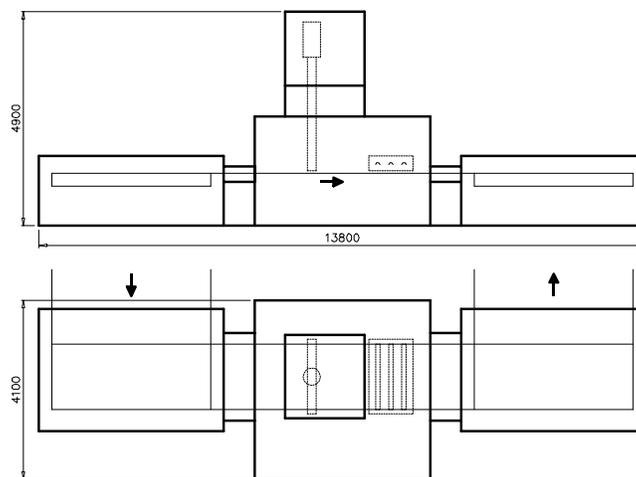
Fig. 4: Electron-beam equipment for boards application (schematically).
