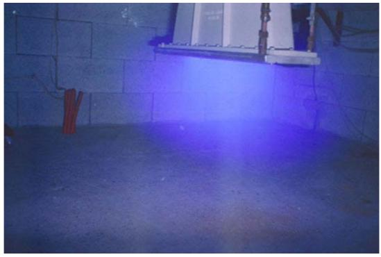
Fig. 2 Excitation of electrons in gas,  $U_B = 230 \text{ kV}$
