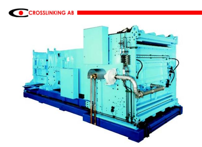
Fig. 4 EB-unit for irradiation of material from roll to roll with drum for web guidance
