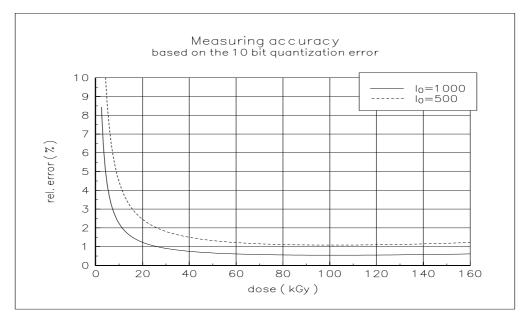
With a dose of 40 kGy and a measured intensity of 1000, the relative quantization error is 0.75 %. With the same dose and a measured intensity of 500, the relative quantization error is 1.5 %.
