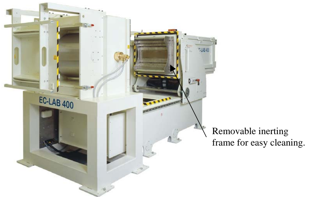
Fig. 15. EC-LAB 400 unit with combined batch and roll-to-roll features in service position.
