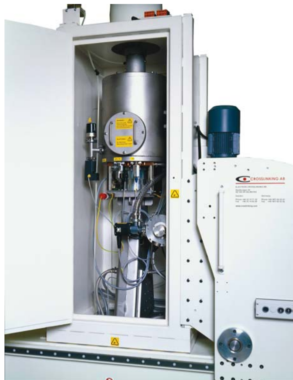
Fig. 11. EC-LAB 400 accelerator with pump system (80 – 300 kV, 5-30 m/min, 400 mm).
