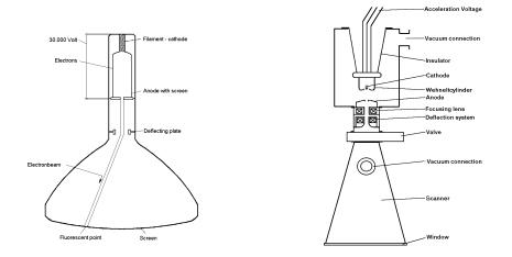
Fig. 1.: Cathode ray tube and the Electron Crosslinking electron beam accelerator
