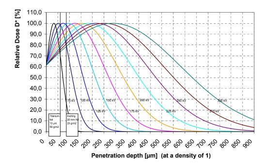
Fig 3.: Range of penetration with different accelerating voltage 13  $\mu m$  titanium foil and 20 mm of Nitrogen. [22]
