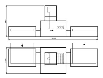
Fig. 4: Electron-beam equipment for boards application (schematically).
