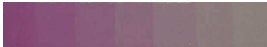
Figure 12. Irradiated dosimeter film 10 µm
